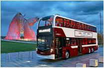
The 3-axle buses on a Volvo B8L chassis will be super-efficient, not least thanks to an electric power train and battery, and the fact that they have passenger doors in the middle as well as at the front. However, they still run on diesel.
