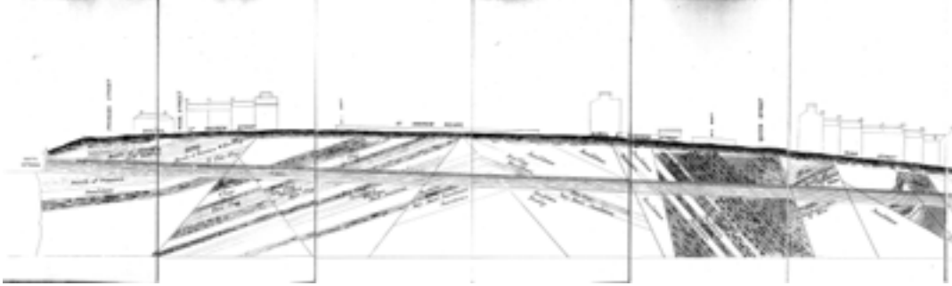
FIG 9 Paterson, 1846. Geological Section through the length of the tunnel (southern half). [Bound drawing, Edinburgh Room, Edinburgh Central Library]
